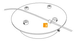
4 Reinstall rubber strain relief bushing with COAX. Tighten down on the strain relief screw securing the fixture and COAX at its desired length.
