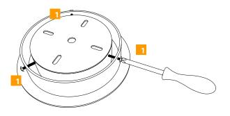
2 Loosen strain relief screw releasing the rubber strain relief bushing.
